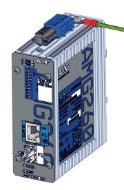
To provide correct protection from ESD and Surge events ensure that the unit is correctly earthed using the provided earth connection point in accordance with local electrical codes & standards. (cable not provided)
